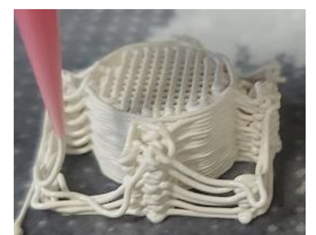
Figure 4. Structure 3D-printed using the LTO paste.
